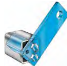
Inner square with through holes and bolted-on lever arm
